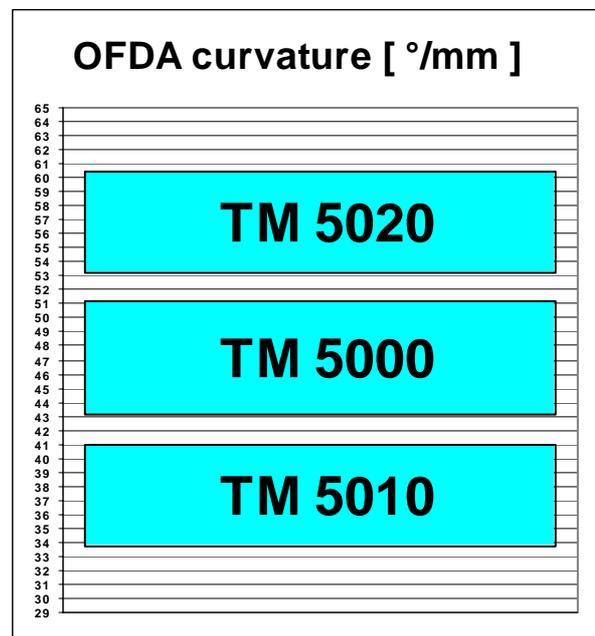
Using OFDA it is possible to define the specification ranges for the different crimping levels - an advantage which must be made use of. A real improvement with regard to quality consistency is then possible with tangible results.
