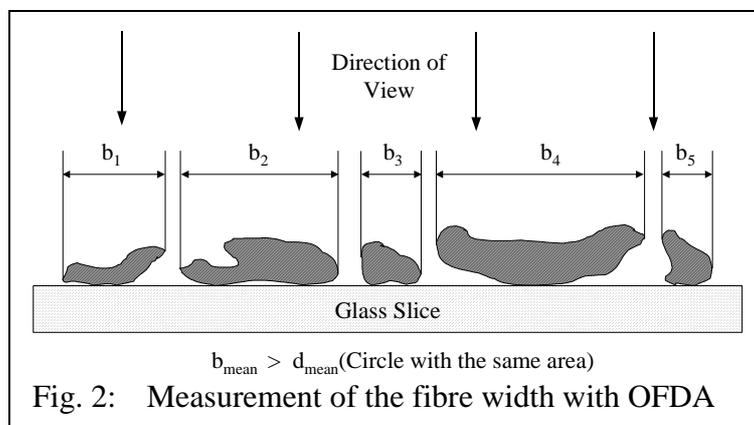
Fig. 2: Measurement of the fibre width with OFDA
